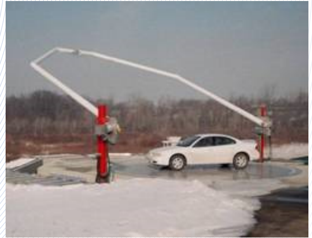
Outdoor Telematics Measurement System
