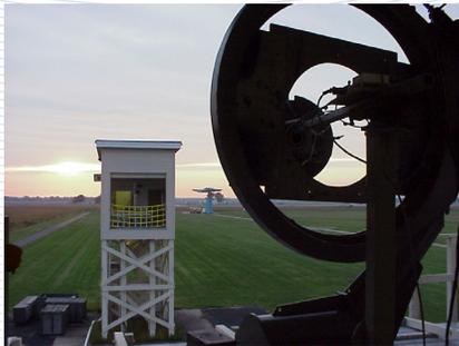
The test positioner axes are controlled and read out by the position control and readout units. A typical control system consists of a control unit located in the operator's console. It is interfaced to a power amplifier unit located near the test positioner. This configuration keeps the high power drive signals near the positioner and away from sensitive measurement instruments while providing remote control of positioner functions from the equipment console.
